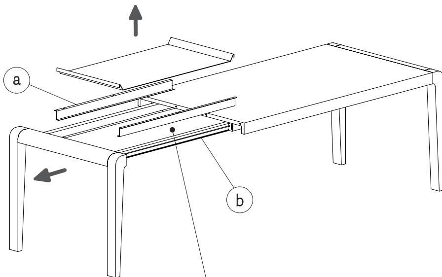
**EN** - 2) Place the metal components (a) as shown and mark the position of the hole on the two extensions (b).
