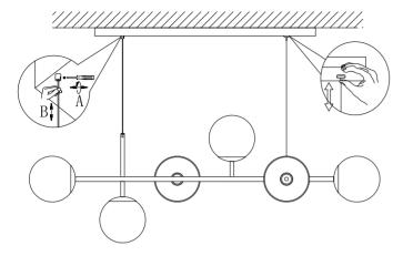
when adjusting the length of the wire, please note to press the button at the canopy in order not to damage the wire
