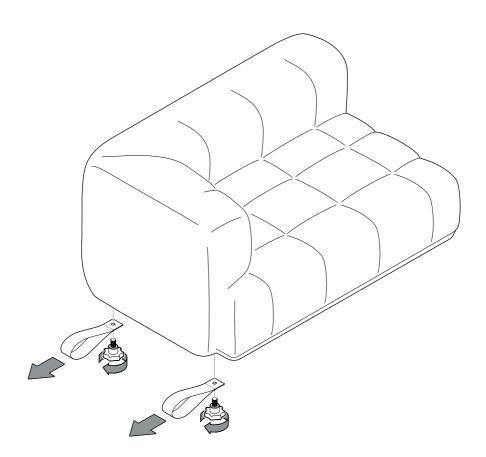
To lock two modules together, connect the fittings by interlocking them as illustrated. Once they are connected together, give the module an extra push to make sure it is firmly locked in place.
